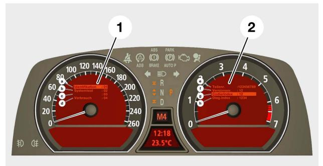
The instrument cluster of the E65 has 21 test functions that can be read out of the LCD display areas 1 and 2.
